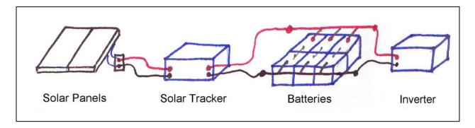
Minimum Connecting Wire Size Recommendations: Copper Only, 12 AWG or 2.6 mm.
