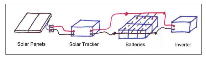
Minimum Connecting Wire Size Recommendations: Copper Only, 2 AWG or 8 mm.
