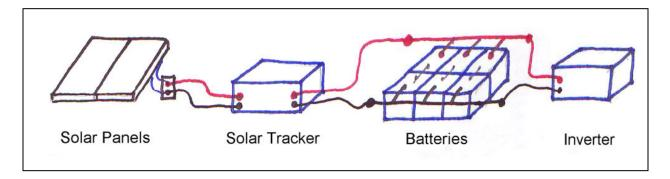
Minimum Connecting Wire Size Recommendations: Copper Only, 6 AWG or 5 mm.
