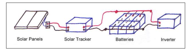
Minimum Connecting Wire Size Recommendations: Copper Only, 4 AWG or 6 mm.
